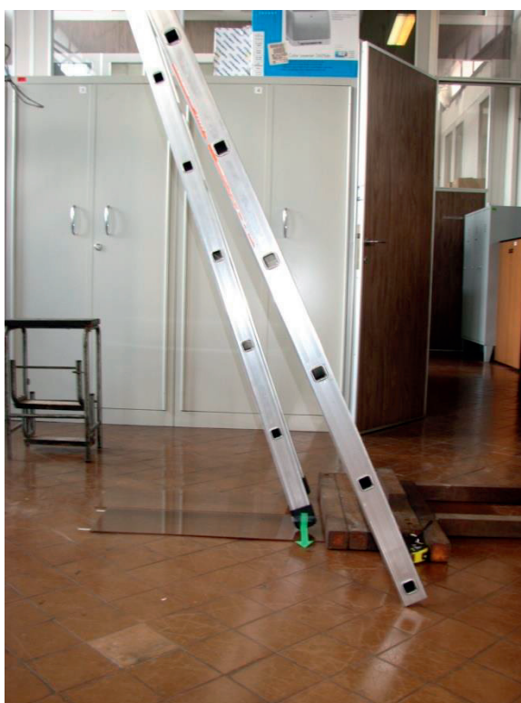
Figura 4.2.1-6 Scale inclinate a 65° e 70°
