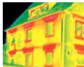
Building with heat loss
